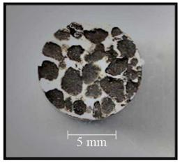
Figure 4: Cross-sectional image of a bed of pellets made of graphite, NaF salt, and water, then infiltrated with molten Vit106. Sample density is 3.91 g/cm<sup>3</sup> (relative density57.4%).
