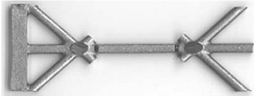
Fig. 3—Photograph of strut sample for tension testing. The long face strut is the gage and the adjacent nodes and face struts are used for gripping.
