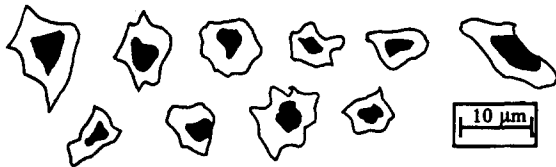
Fig. 10. Outlines of particles and their associated plastic zones traced by hand from enlarged micrographs. There is no correlation between the shape of a particle and that of its plastic zone.
