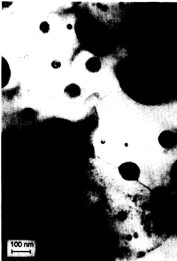
Fig. 7. TEM image of NiAl-10W HIPed at 1200 ^{\circ}\text{C} .
