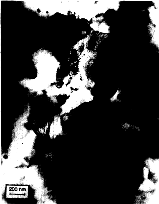
Fig. 5. TEM image of NiAl-10Mo synthesized by the intermetallic route and HIPed at 1000 °C.
