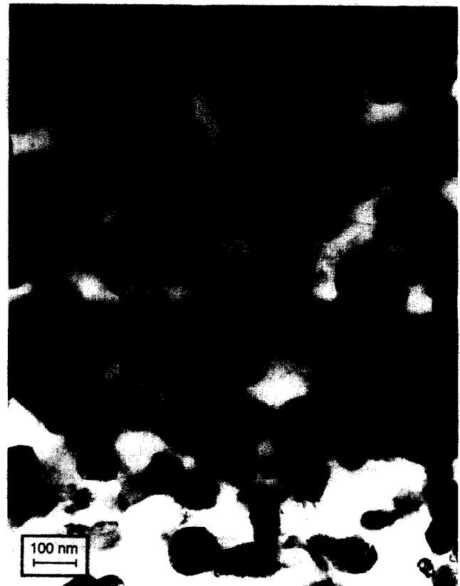
Fig. 8. TEM image of NiAl-30W HIPed at 1000 ^{\circ}\text{C} .
