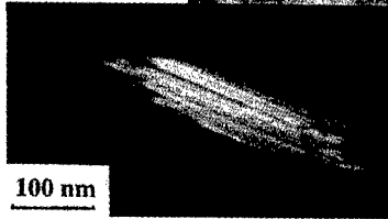
Figure 5, Dark field TEM image of the 0.5 % B 900 °C HIPed material showing the growth faulting of the needle precipitates.
