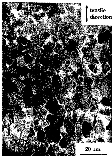
Figure 6, Backscattered SEM image showing cavitation in a milled Ti-6%Al-4%V sample HIPed at 700 °C and tensile tested at 900 °C and 6 \times 10^{-4} \text{ s}^{-1} .
