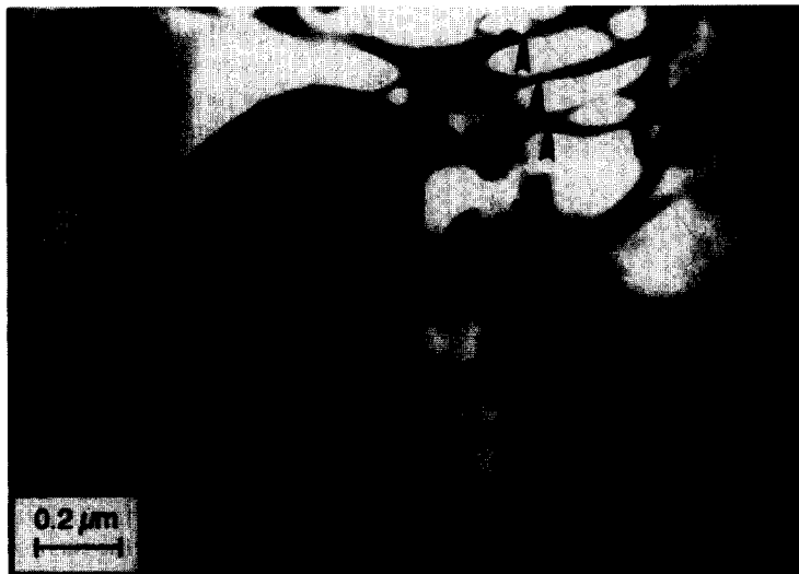
Fig. 4. (a)–(c) TEM micrographs of extruded, fine-grained DSC-Al crept at 450°C under a stress of 33 MPa and cooled under load showing pile-ups of dislocations (arrows) interacting with alumina dispersoids (A).
