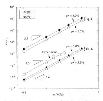
Fig. 10—Compressive strain rate vs stress plot at 900 °C showing experimental data for 20 ppi foams ( $\rho^* = 5.0$  to 5.5 pct) and predictions of analytical models assuming creep bending of struts (Eq. [4]) or creep compression of struts (Eq. [6]) for  $\rho^* = 5.0$  and 5.5 pct.
