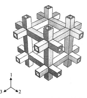
Fig. 4—Geometric FEM models for foam with hollow struts ( $\rho^* = 5.0$  pct). In the solid-strut model, struts have smaller width but the same cross sectional area.
