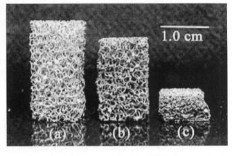
Fig. 1—20 ppi NiAl foam (*a*) as-processed, (*b*) deformed by approximately 20 pct at 0.8 MPa at 900 °C, and (*c*) deformed by approximately 70 pct at 1.5 MPa at 900 °C.
