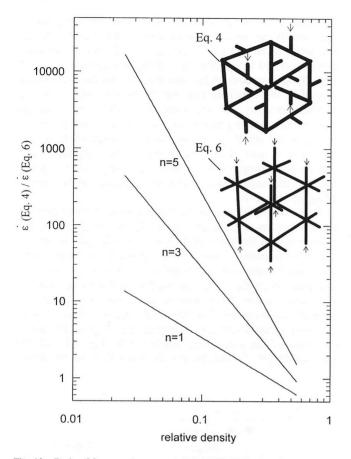
Fig. 12—Ratio of foam strain rates predicted with the creep-bending model (Eq. [4]) and the creep-compression model (Eq. [6]), as a function of relative density; the ratio is independent of temperature.
