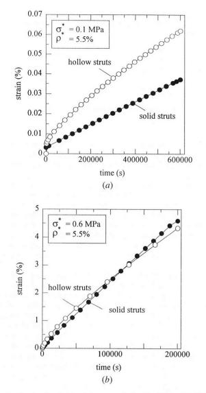
Fig. 5—Compressive strain vs time curves calculated by FEM at 900 °C for foams with hollow and solid struts ( $\rho^* = 5.5$  pct) at stresses (a)  $\sigma^* = 0.1$  MPa and (b)  $\sigma^* = 0.6$  MPa.
