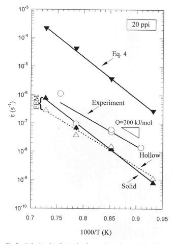
Fig. 8—Arrhenius plot of creep data for experimental tests on 20 ppi foams ( $\rho^* = 5.0$  to 5.5 pct,  $\sigma^* = 0.22$  to 0.25 MPa) and FEM predictions ( $\rho^* = 5.5$  pct,  $\sigma^* = 0.25$  MPa).
