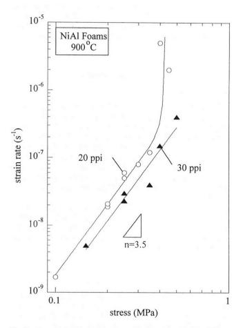
Fig. 3—Compressive strain rate vs compressive stress for 20 ppi foams ( $\rho^* = 5.0$  to 5.5 pct) and 30 ppi foams ( $\rho^* = 6.6$  pct) at 900 °C.
