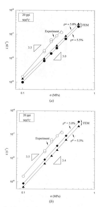
Fig. 6—Compressive strain rate vs stress curves at 900 °C as measured experimentally on 20 ppi foams ( $\rho^* = 5.0$  to 5.5 pct) and as calculated by FEM ( $\rho^* = 5.0$  and 5.5 pct) for (a) hollow struts and (b) solid struts.
