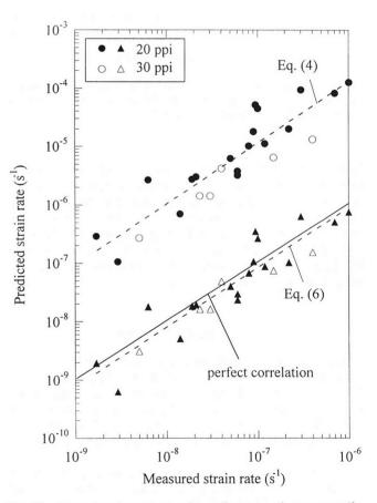
Fig. 11—Comparison between experimentally measured creep rates (for 20 and 30 ppi foams between 800 °C and 1100 °C) plotted on the *x*-axis and creep rates predicted from analytical models plotted on the *y*-axis (1) assuming creep bending of struts (Eq. [4], circles show a discrepancy by a factor of approximately 100 from perfect correlation) and (2) creep compression of struts (Eq. [6], triangles show a discrepancy by a factor approximately 2). Dotted lines are best-fit regressions.
